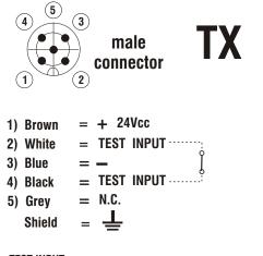
$\begin{array}{l} \textbf{TEST INPUT} = \text{Opening contact TEST INPUT (PIN2/4) is simulated} \\ \text{the interruption of the curtain and testing the correct opening} \\ \text{of the outputs SW1 - SW2 of the receiving unit} \end{array}$
